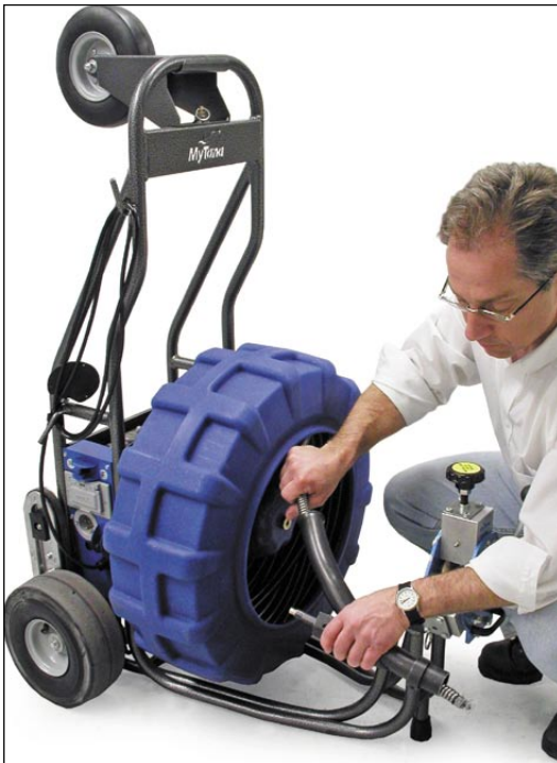
Slide the automatic feed out by pulling down on the ring pin. Feed cable through the revolving arm.
