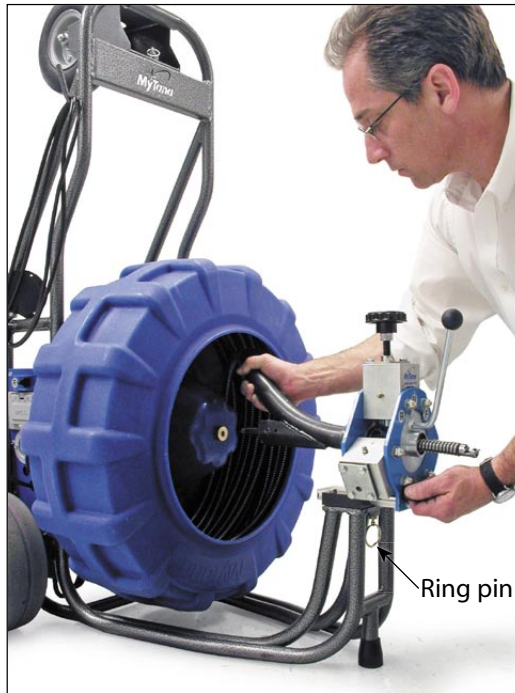
Insert the cable through the automatic feed. Place the revolving arm into the autofeed, pull down on the ring pin and slide the autofeed towards the reel so the revolving arm fits into the reel unit. Make sure the ring pin snaps into place.
